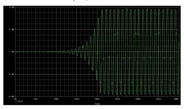
Replacing  $R_2$  with 13  $k\Omega$  pot and two Schottky diodes between the wiper and node 3, with 6.4  $k\Omega$  between the diodes results in a sinewave with an amplitude of approximately 2V:
