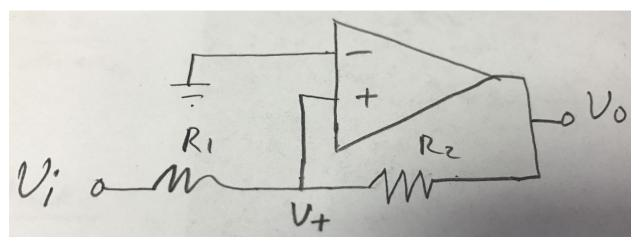
The op amp circuit is in a positive feedback configuration.
