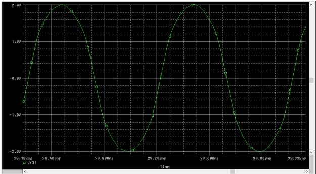
How high in frequency can this oscillator go? All C's were replaced with 159.16pF, which should result in a 999,969 Hz (almost 1 MHz) sinewave.
