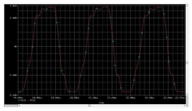
The distorted sinewave has a fundamental frequency of approximately 950 KHz. The oscillator used the 25 MHz GBW product AD8610 op amp for all op amps. The distortion might also be due to the AGC diodes.
