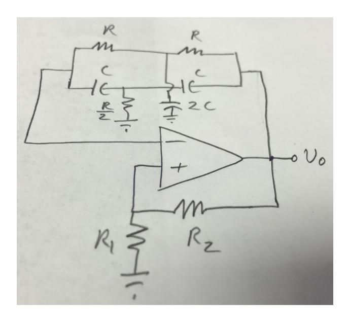
The op amp circuit is unstable due to positive feedback. However, the twin T network provides negative feedback except at  $\omega_o$ , which stabilizes the circuit at other frequencies. At  $\omega_o$ , the op amp circuit is unstable due to positive feedback, and oscillates at that frequency.
