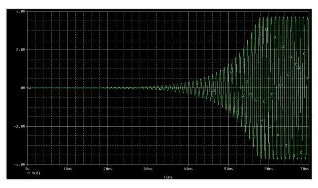
AGC:  $R_2$  replaced with a 10  $k\Omega$  pot, two 0.5V Schottky diodes connected between the wiper and one end, in opposite directions. The pot is set with 5  $k\Omega$  on each side of the wiper:
