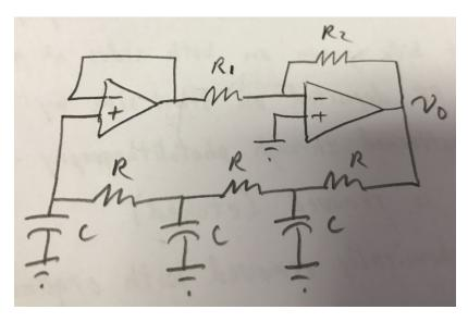
$$A(j\omega)\beta(j\omega) = \frac{-\frac{R_2}{R_1}}{(sCR)^3 + 5(sCR)^2 + 6sCR + 1}$$
