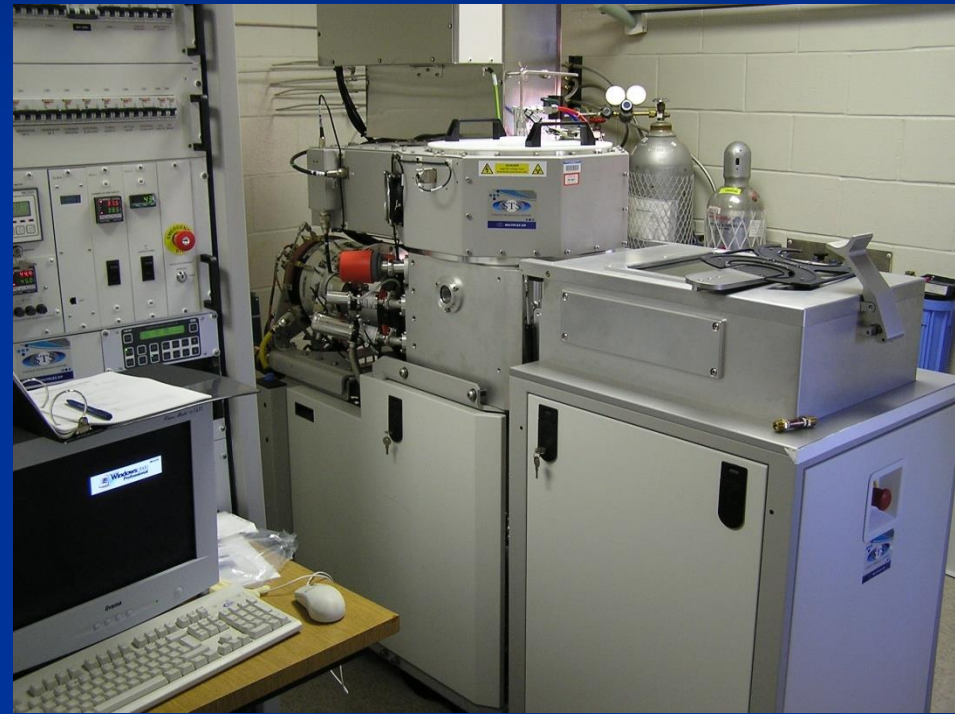
STS ASE Bosch Process Si DRIE Etcher
