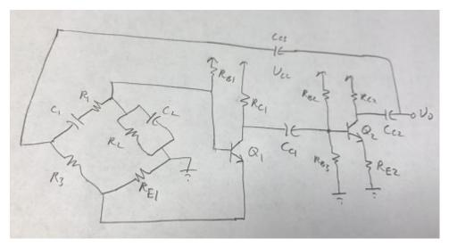
This circuit uses a two stage amplifier (two negative gain common emitter amplifiers) to achieve a positive gain for the Wein bridge oscillator.
