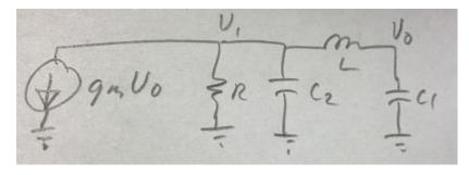
From this tank circuit configuration, we know that:  $\omega_0 = \sqrt{\frac{C_1 + C_2}{LC_1C_2}}$
