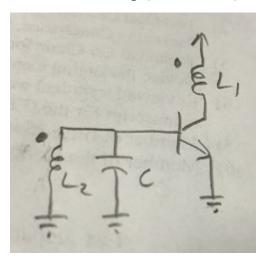
Without biasing resistors shown. The transformer provides feedback from the output of the common emitter amplifier back around to the base. A transformer can easily provide a 180° phase shift. Transformer's inductance with C determines the oscillation frequency.
