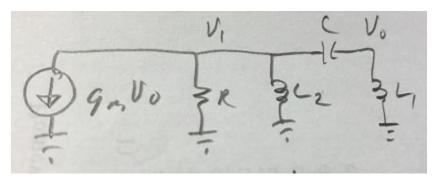
Here, the tank circuit has  $\omega_o = \frac{1}{\sqrt{C(L_1 + L_2)}}$
