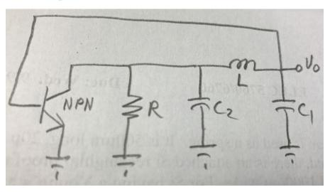
Notice that the biasing resistors are not shown in this simplistic circuit.
