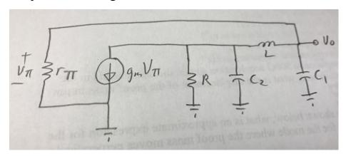
Let's further simplify by assuming that  $r_\pi$  is so large that we can approximate  $r_\pi$  as an open circuit:
