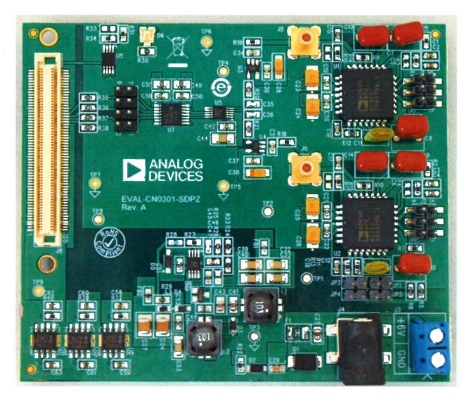
AD698 LDVT Signal Conditioning Subsystem
