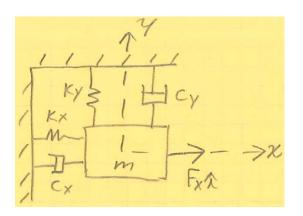
$F_x = A_x \sin(\omega_d t) \rightarrow \text{to force m to oscillate along x-axis (using an actuator)}$
