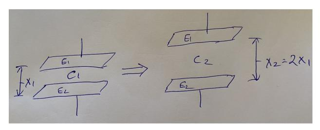
$E_1$  and  $E_2$  are two parallel plate electrodes used to form  $C_1$  and  $C_2$ , respectively. For  $C_1$ , the electrode separation distance is  $x_1$ , and for  $C_2$ , the electrode separation distance is  $x_2$ , where  $x_2$  is twice the distance of  $x_1$ . It is assumed that the electrode area is much greater that the electrode separation distance squared, so that fringing effects can be neglected.
