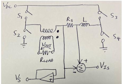
A controller (microcontroller, FPGA, etc.) uses  $V_s$  and  $V_{Is}$  in adjusting the two PWM signals:  $V_s$  is proportional to  $V_{OUT}$  and  $V_{Is}$  is proportional to the current through  $R_s$ . A temperature sensor could also be included so that the controller can shut off the inverter if it begins to overheat.
