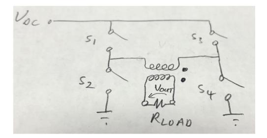
The transformer also provides DC isolation between the input DC source and the load, which can be very important in protecting the load if a transistor switch fails, since transistors often fail in a state where they are permanently turned on.
