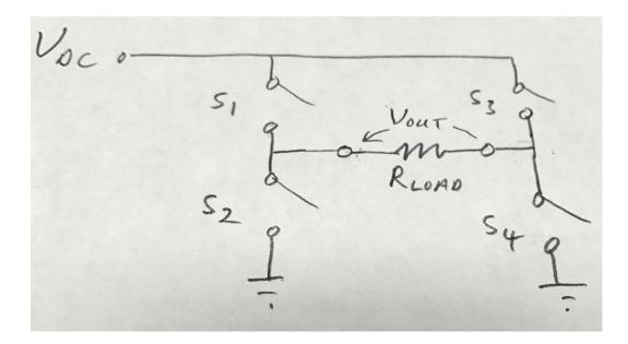
The four switches are power transistors (MOSFETs, IGBTs, BJTs, etc.). They need to be sufficiently fast (turn on / turn off times), low on-resistance, able to handle sufficiently high voltages and currents, and are properly heat sinked. This configuration is called an H-bridge,
