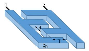
It consists of two interdigitated comb-style electrodes. One electrode is considered as fixed in space. The other one is secured by a suspension system that only allows it to move such that its teeth can move in or out of the teeth of the other electrode.
