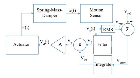
The RMS block determines the root mean square value of the  $V_s$  signal,  $V_{rms}$ . This signal is compared with a reference voltage,  $V_{ref}$ , which generates an error signal if they are not equal. The integrator and multiplier attempt to reduce  $V_{error}$  to 0 V by keeping the amplitude of x(t) at the desired value. The integrator is necessary to reduce the error in the proof mass amplitude to zero.
