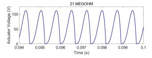
Since MEMS devices can operate over a much larger temperature range than semiconductor electronic devices, the DC source – resister – PPA MEMS resonator could be used to generate AC voltage signals in operating environments too hot or too cold for transistors to operate.
