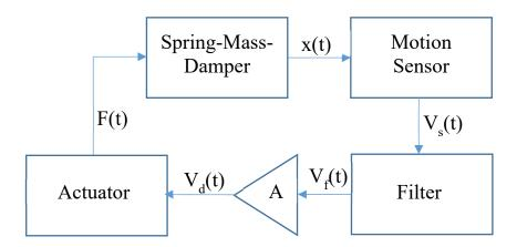
where all of the components are approximately linear and the system satisfies the Barkhausen criterion for oscillation. When examining the components, it is important that they also have (or approximately have) a linear response:
