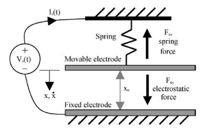
Force is proportional to voltage squared and inversely proportional to electrode separation distance squared. The PPA's response is highly nonlinear.
