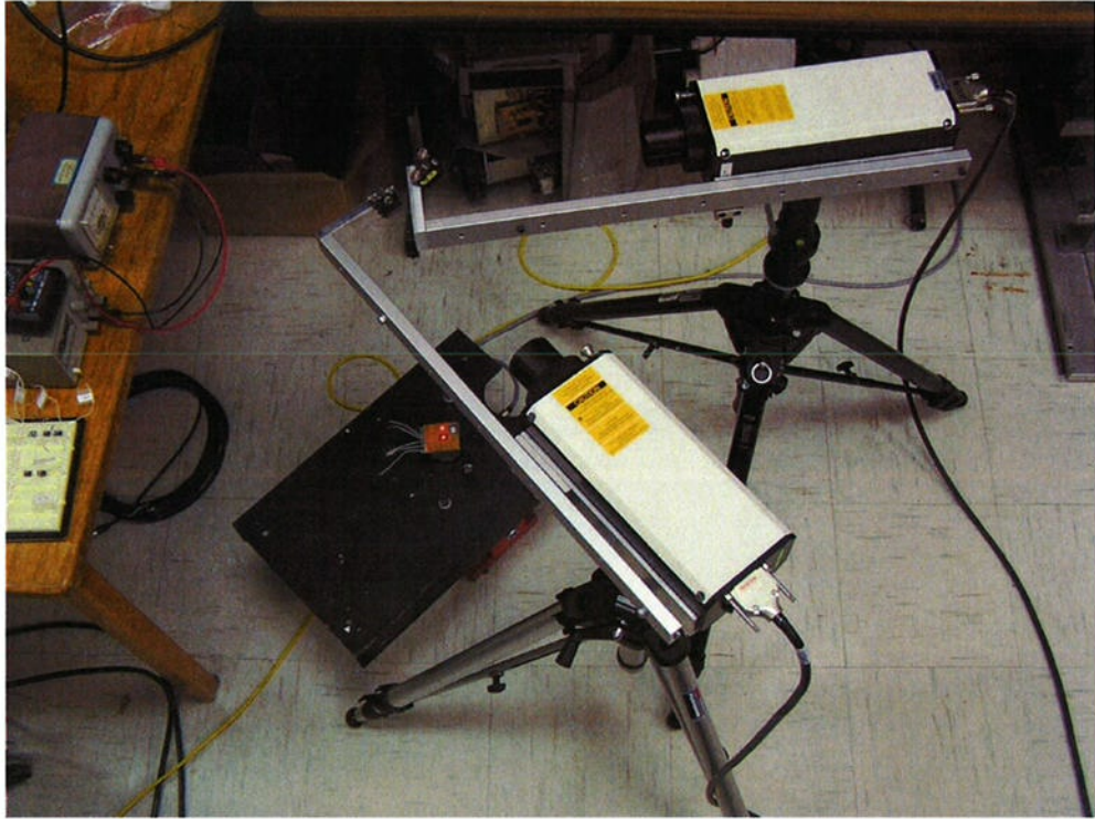
2 laser interferometers used to measure transmissibility of MEMS device on shaker
