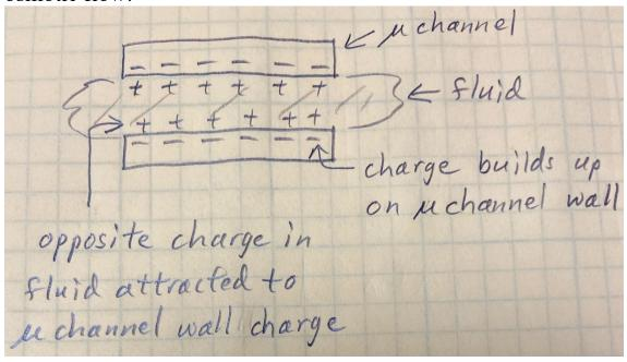
The charge buildup on the sides of the  $\mu$  channel is like that previously discussed with metal electrodes in water where an electrical double layer forms on them.
