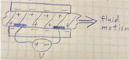
A voltage of around 100 V across the two electrodes is sufficient to cause fluid flow. DMOS transistors exist that operate at that voltage level:
