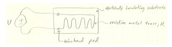
Power dissipated in R by heat:  $P = i^2R \rightarrow \text{called Joule heating}$ .
