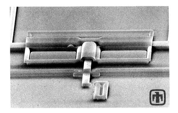
b. Internal Combustion Engine on a Chip
