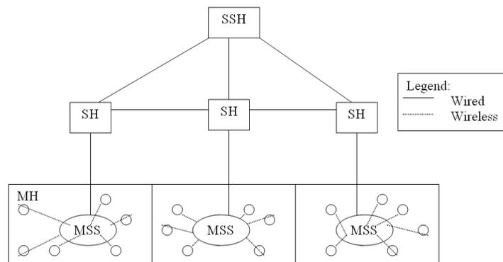
**Figure 1:** Four-layered Mobile Cellular Network Architecture
