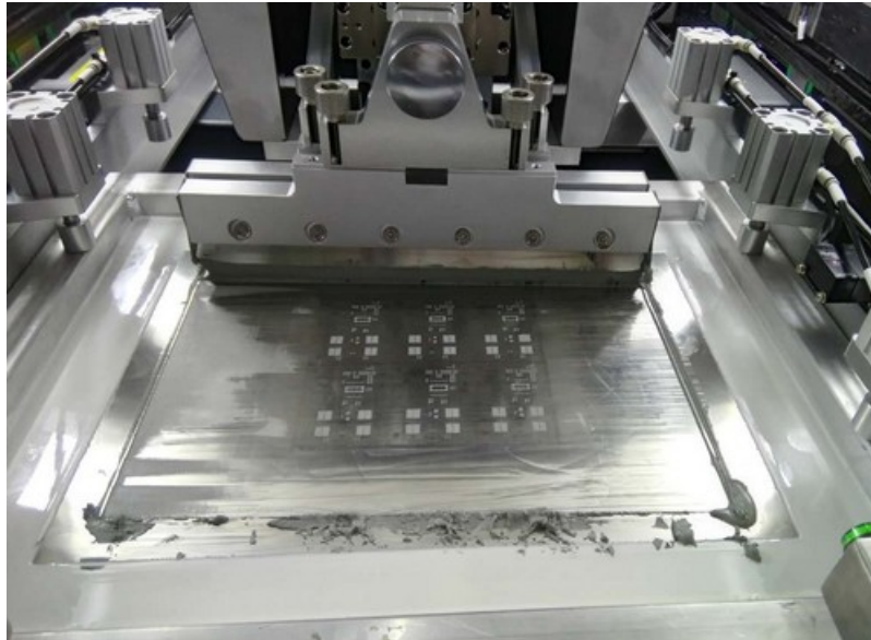
Figure 2.22: Solder paste printing process [17].
