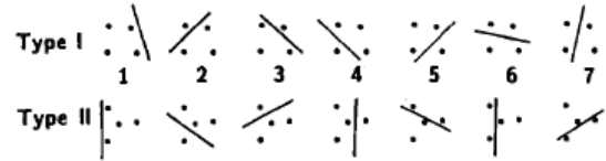
Fig. 2. Classification of target trajectories according to the way of sensor field decomposition.
