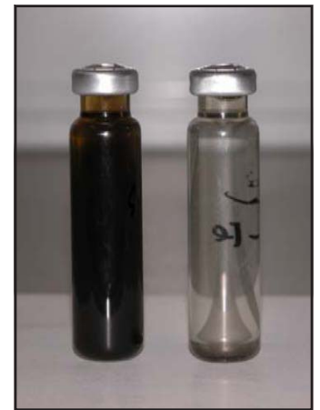
Visual comparison of nanoparticle stability after five days: stabilized (left) vs. unstabilized (right)
