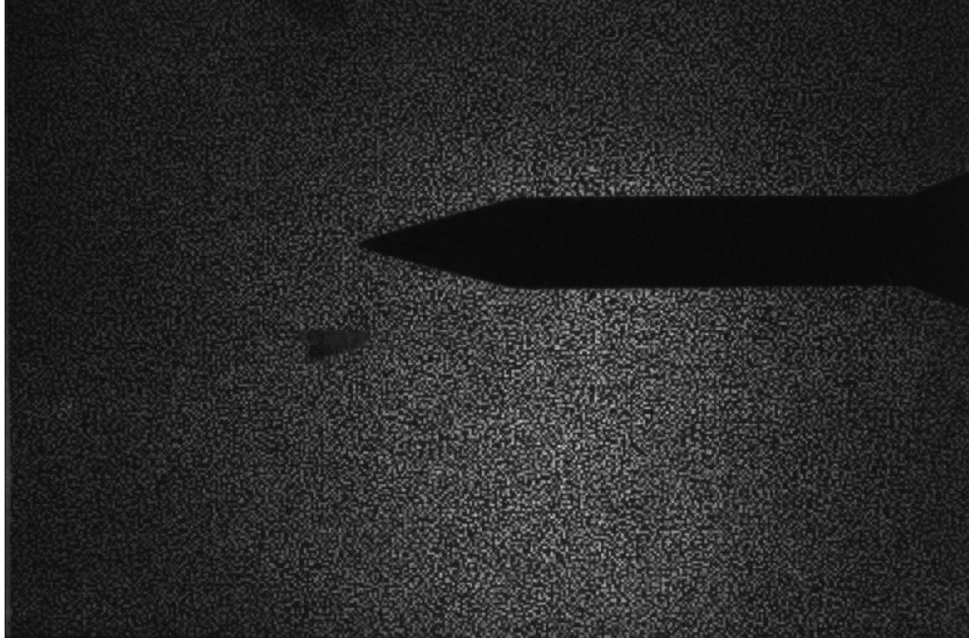
Figure 11. Raw image of the cone model in Mach 2.0 flow.
