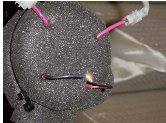
Figure 3: Photograph of the plasma arc used for 3-D array calibration.
