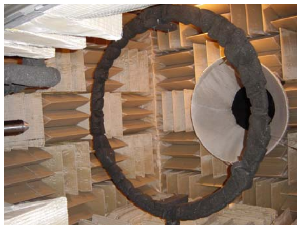
Figure 2: Photograph of the 3-D microphone array within the optically accessed anechoic chamber of the Gas Dynamics and Turbulence Laboratory.
