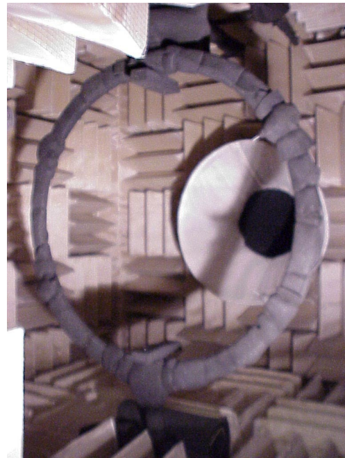
Figure 5: Picture of the arc array in the anechoic chamber. It has been wrapped in acoustic foam.
