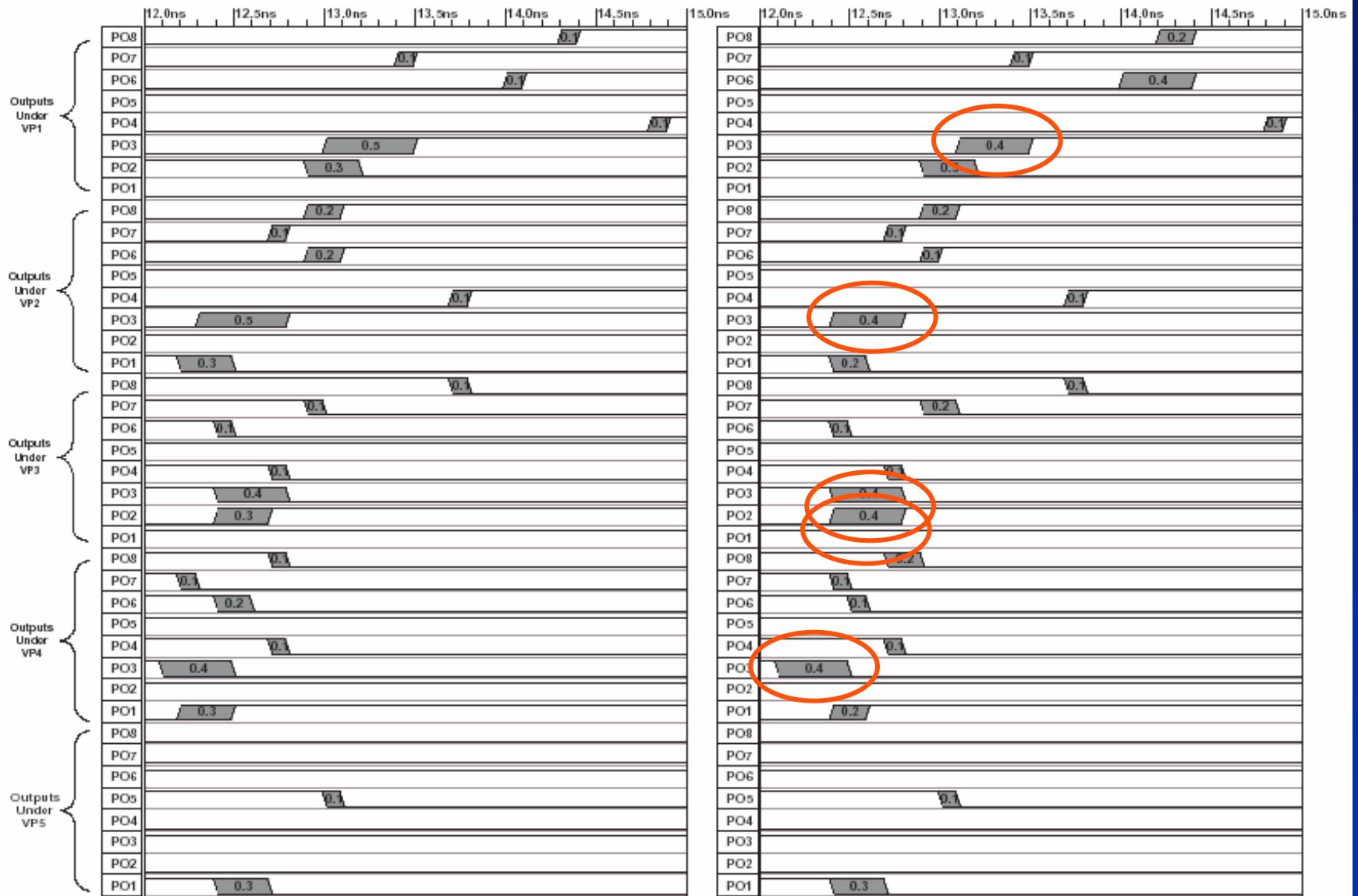
(a) Output transitions of experimental chip1 for five test vector pairs
