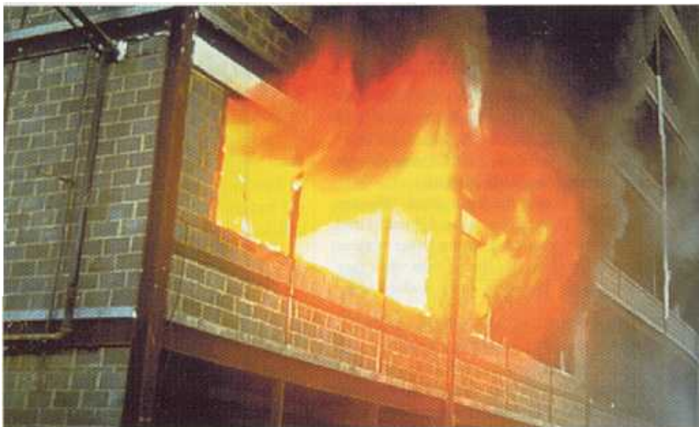
View of Cardington Test Building during fire exposure.
