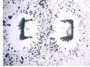
Magnetic field in a bar magnet
