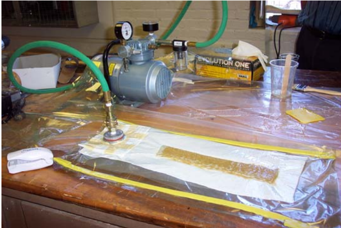
Figure 5 Composite manufacturing with vacuum bagging technique
