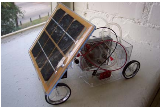
Figure 2. Fuel cell car with solar panel (left); production of hydrogen from distilled water using a lamp and the solar panel.
