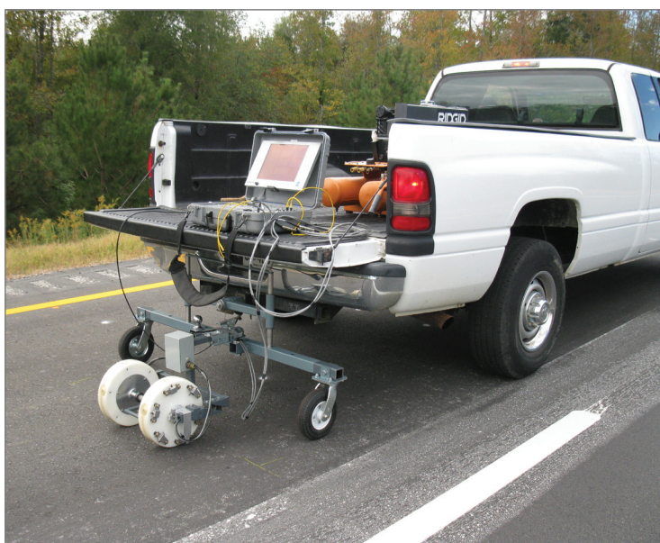
Figure 3. Seismic wave technology used in field evaluation at the test track
