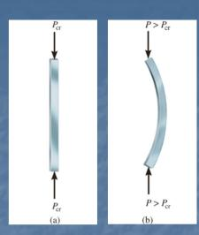
$P_{cr}$  = critical axial loading (maximum axial load that a column can support just before it buckles)
