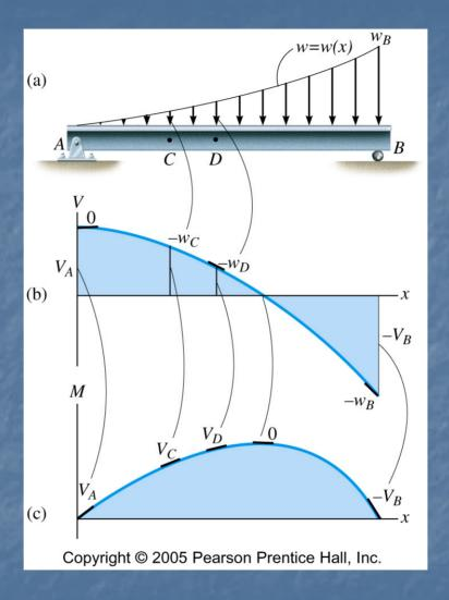
Slope of shear diagram = negative of distributed loading value  $\Rightarrow -\frac{dV}{dx} = q(x)$ Slope of moment diagram = shear value  $\Rightarrow \frac{dM}{dx} = V$
