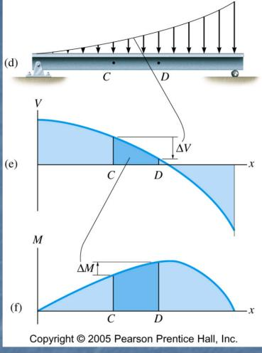
Change in shear between two points = neg. of area under  $V_2 - V_1 =$  distributed loading diagram between those two points  $\rightarrow$
