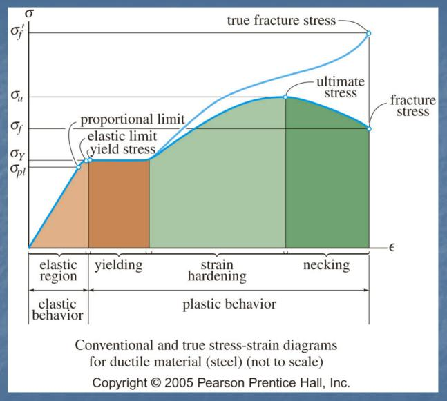
Stress-Strain Diagram for Normal Stress-Strain
