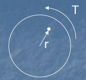
r = distance from center to point of interest in cross-section (maximum is the total radius dimension)
