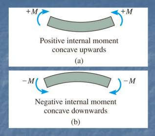
Inflection point is where the elastic curve has zero curvature = zero moment
