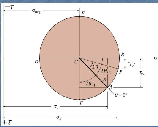
A rotation of  $\theta$  to the x' axis on the element will correspond to a rotation of  $2\theta$  on Mohr's circle!
