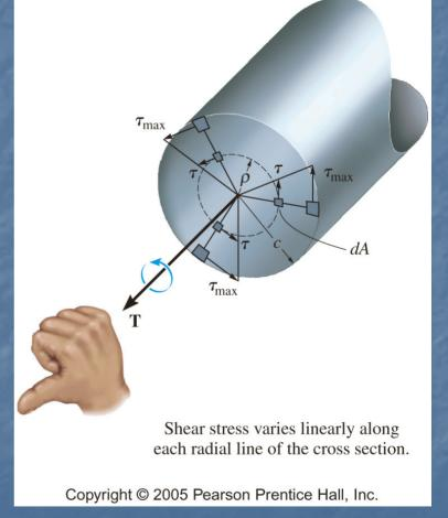
Shear stress,  $\tau$ , and shear strain,  $\gamma$ , vary linearly from 0 at center to maximum at outside of shaft
