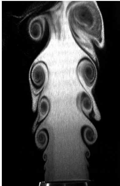
Fig. 7 – a) Instantaneous and b) Average image of the acoustically excited jet with f=30\text{Hz} , V = 7.3 \text{ ft/s} , St = 0.426
