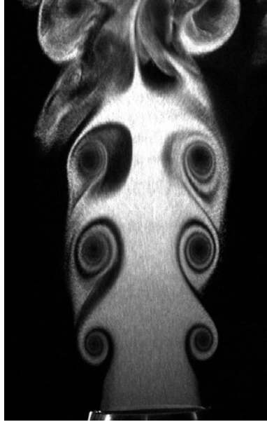
Fig. 6 Instantaneous image of the acoustically excited jet with f=30\text{Hz} , V = 5.5 \text{ ft/s} , St = 0.738
