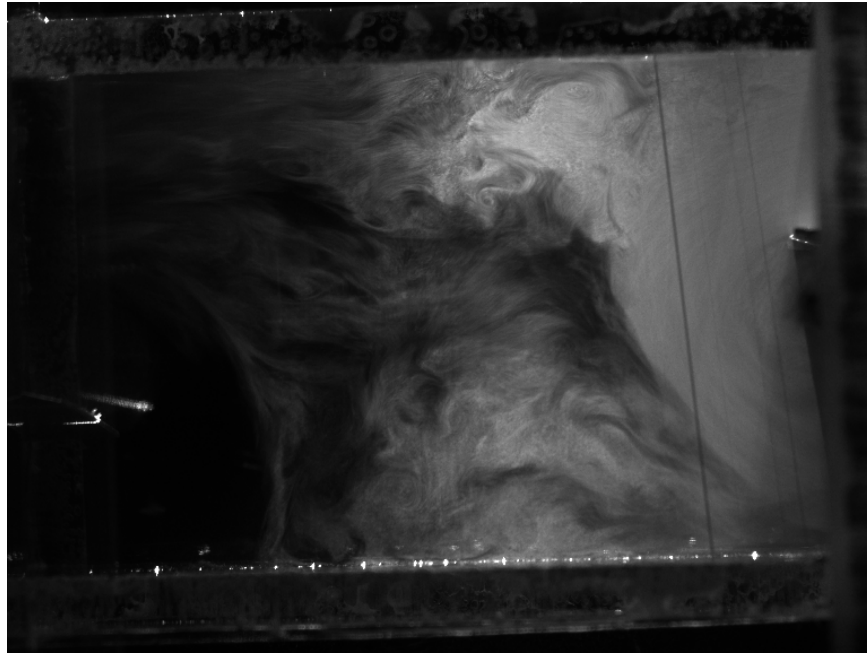
Fig. 8 Splitter plates are at a 0.625 inch separation in the plates with a free stream velocity of 11.5 feet per second
