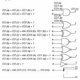
The sequential testability measures are incremented only when they pass through a Flip-flop.
