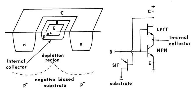
A TRIPLE DIFFUSED NPN BIPOLAR TRANSISTOR WITH SIT PROTECTION
