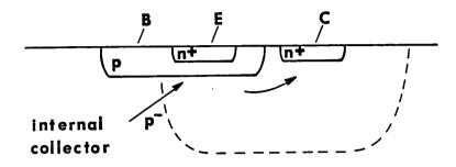
\* A MODIFIED BIPOLAR STRUCTURE FOR VLSI
