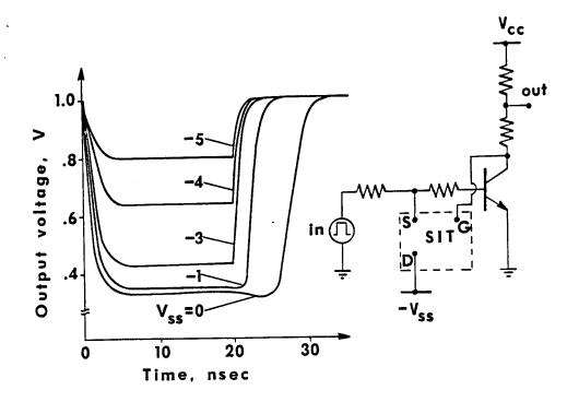
\* OUTPUT WAVEFORMS FOR A CHAIN OF INVERTERS WITH SIT PROTECTED BIPOLAR TRANSISTORS
