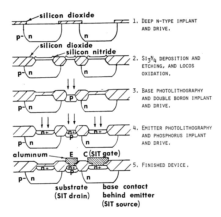
ISOPLANAR PROCESS FOR NPN-BIPOLAR TRANSISTOR WITH S.I.T. PROTECTION AGAINST SATURATION
