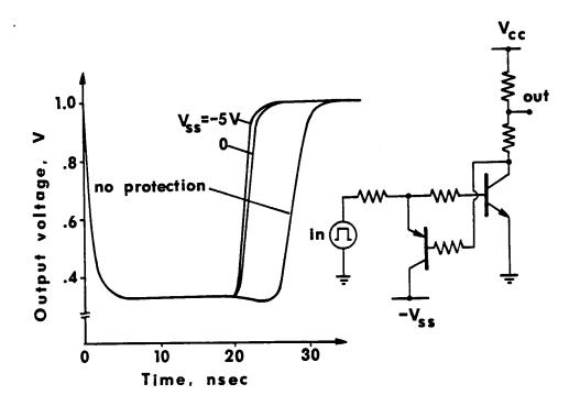
\* OUTPUT WAVEFORMS FOR A CHAIN OF INVERTERS WITH PNP PROTECTED BIPOLAR TRANSISTORS
