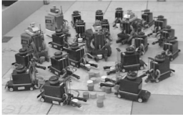
Figure 1: The mobile robots used to demonstrate and verify our group behavior and learning work. These robots demonstrated group avoidance, following, aggregation, dispersion, flocking, wandering, foraging, docking, and learning to forage.
