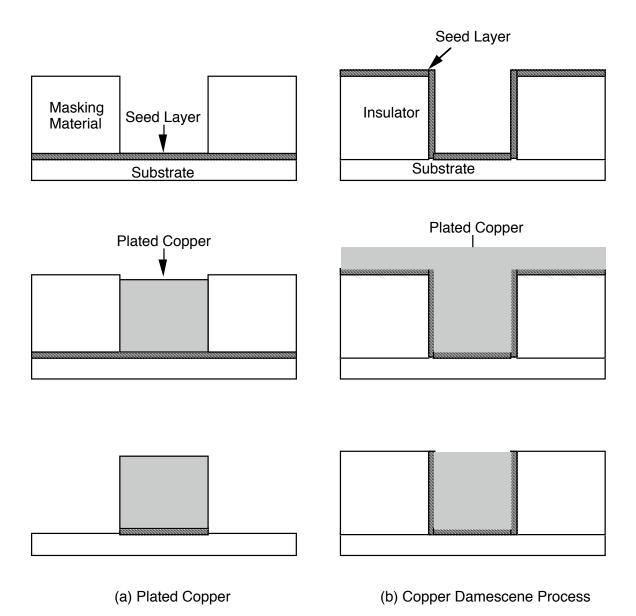
Figure 7.18 - Plated copper and copper Damescene process steps. (a) Mask openings are defined over seed layer and copper is plated in the opening. A nonplanar structure results after plating mask removal. (b) A seed layer is deposited over the patterned insulator, and copper is plated over the entire structure. A planar surface results after the excess copper is lapped away.
