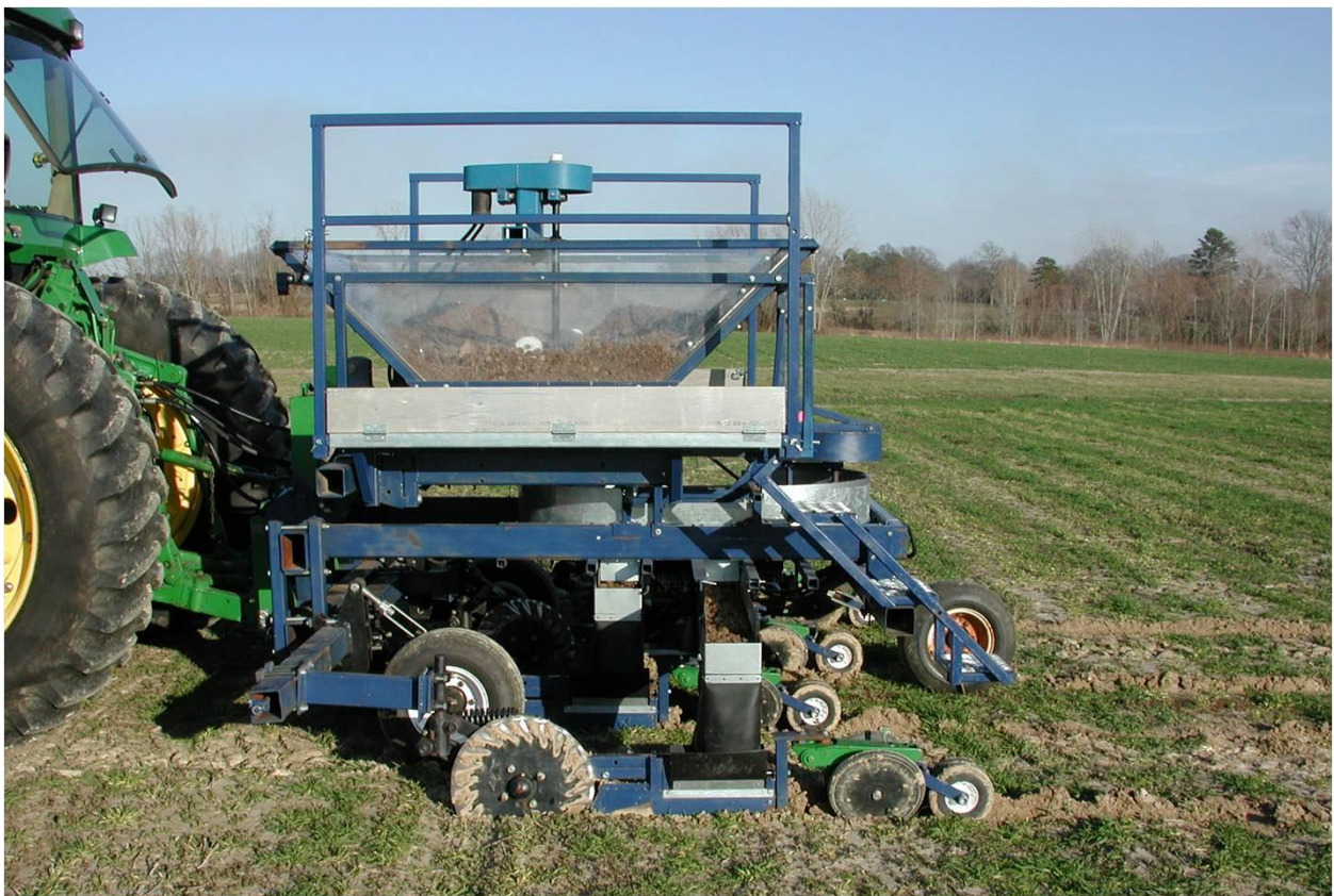
Figure 1- Subsurface Banding Poultry Litter Implement [Way, T. (2010) - Improvement of Soil Trenchers for a Subsurface Banding Poultry Litter Implement (6)]
