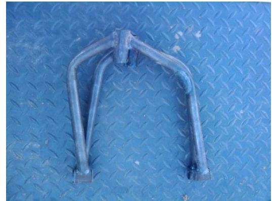
Figure 14- Deformation of upper a-arms
