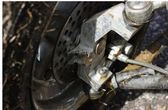
Figure 10-failed front left knuckle at steer mounts
