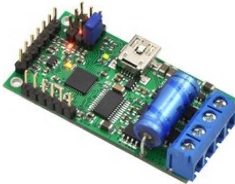
Figure 16 – Motor Controller 24V (Fully Assembled)
