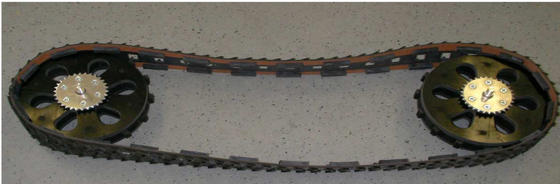
Figure 5.3.5 Combined Tread and Wheel Set
