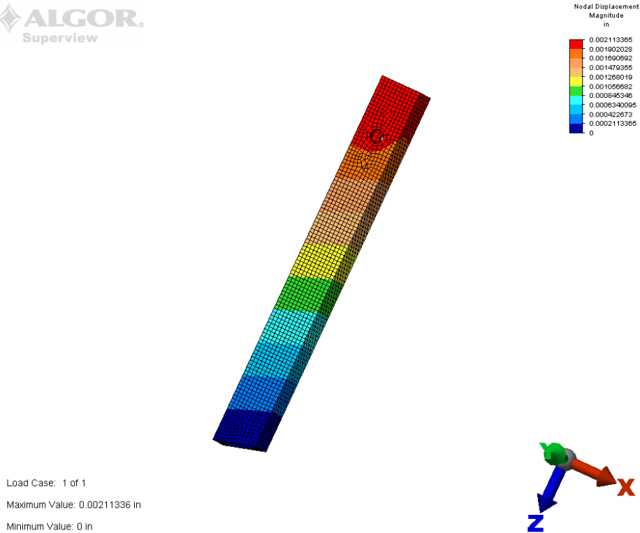
Figure 21: Displacement of front leg insert given worst case scenario
