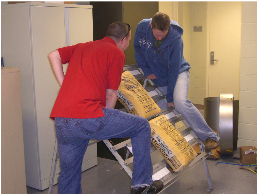
Figure 34: Structural Integrity Testing of Corrosion Stand using Concrete Bags and Personnel
