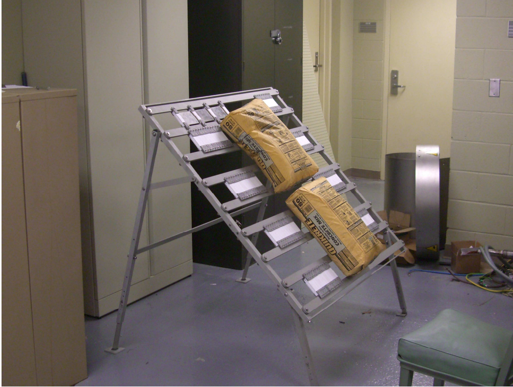
Figure 33: Structural Integrity Testing of Corrosion Stand using Concrete Bags
