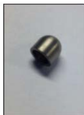
Typical Endcap to Ensure Applied Load at 13mm From Clamping Plane
