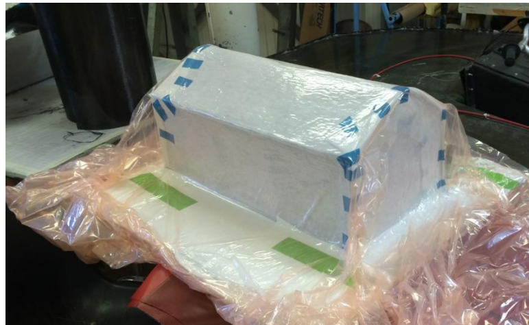
Figure 33: Vacuum Bagging the Bin
