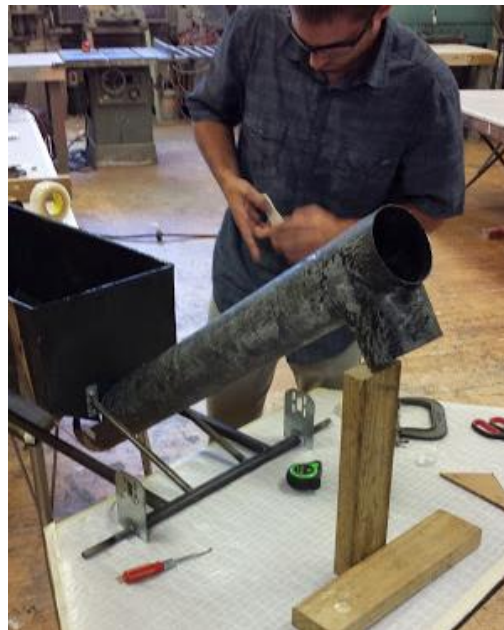
Figure 34: Attaching the Auger Tube to the Bin
