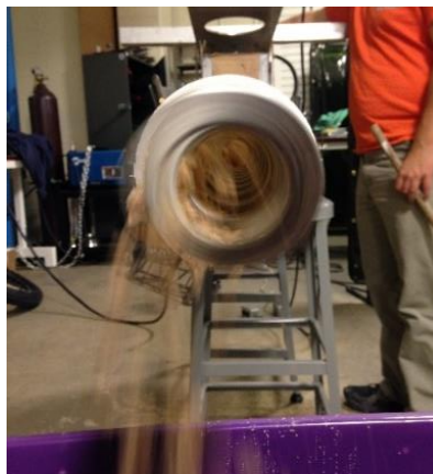
Figure 14: Sand Falling Out of Auger Threads During Testing
