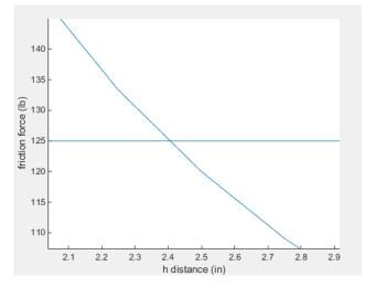
The Clamp design will allow the user to fall at a controlled speed, since the frictional force applied to the rope is proportional to the weight of the user.
