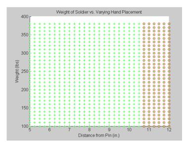
The graph to the right shows that at a distance of 10.75", each user will fall at the same constant speed, regardless of weight. (shown by the red circles ) - This speed is set by the handle geometry and the braking material
